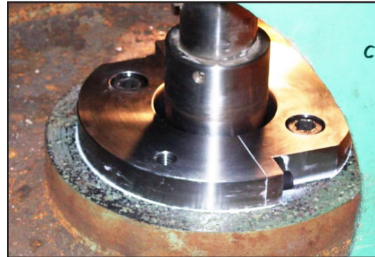
Chesterton 860 MPG cures to form a perfect “form In place” gasket to seal the adapter plate.
