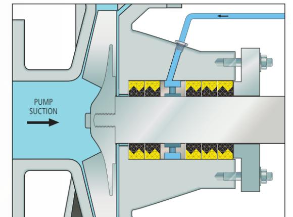
FIGURE 1 – All Rings Oriented for Sealing
