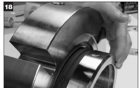
Lift up on the gland and hold the bottom of the sleeve to invert and gently set down to initiate contact between the stationary and rotary faces.
