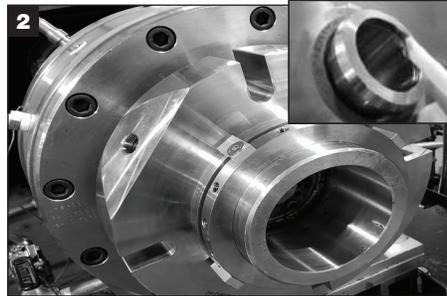
Apply a thin film of **white** grease to the shaft O-Ring (V) and slide seal onto the shaft by pushing on the gland. **CAUTION: Ensure that all set screws are engaged through the sleeve but do not protrude into the sleeve inside diameter bore.**
