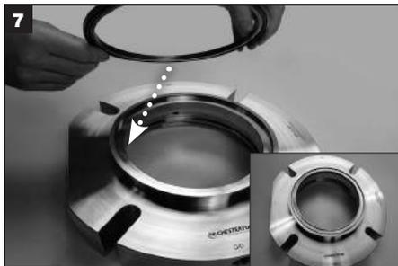
**For seals with Bushing kit:** Install the bushing into the counter bore of the gland with the bushing O-Ring (Y) facing downward.
