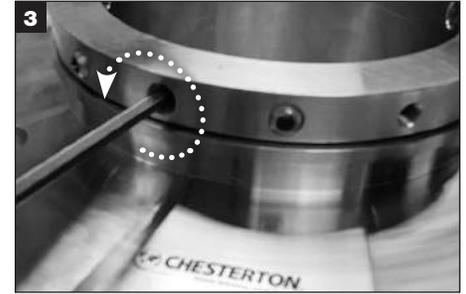
Remove all cup point and dog point set screws from the lock ring and discard.
