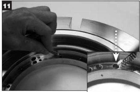
Dip the ends of the springs into white grease and insert into each spring hole. **IMPORTANT: DO NOT** insert springs into the four evenly spaced holes marked by dimples and previously filled with 635 SXC grease.
