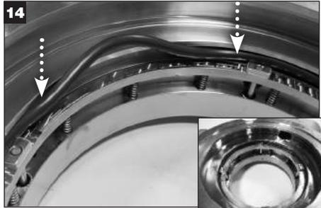
Apply a thin film of **white** grease to the stationary face O-Ring (X) and install into the groove in the gland above the follower plate assembly.
