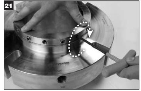
Install the centering clips on the outer diameter of the lock ring with the centering clip flat head screws.
