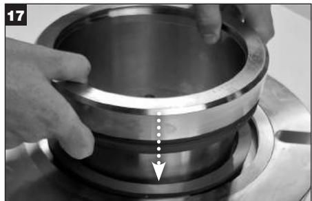
Invert the sleeve assembly and insert it into the gland bore.
