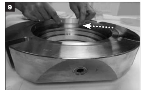
**For seals with Injector option:** Invert the gland. Compress and overlap the ends of the injector, position the splits opposite the F (flush) port and install in the gland groove. **IMPORTANT: The injector should snap into place. Ensure the split ends do not overlap when fully installed.**
