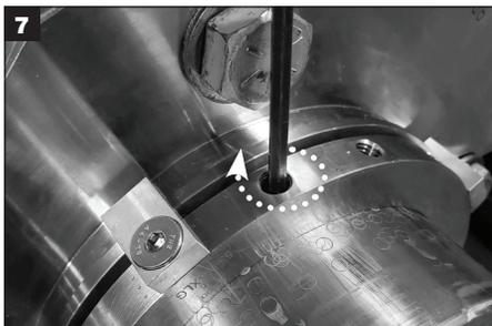
Tighten cup point set screws ② evenly with the hex key provided. **IMPORTANT: After all sets screws have been tightened by hand, retighten with a torque wrench: to 13,6 – 15,3 Nm (120 – 135 in-lbs.)**
