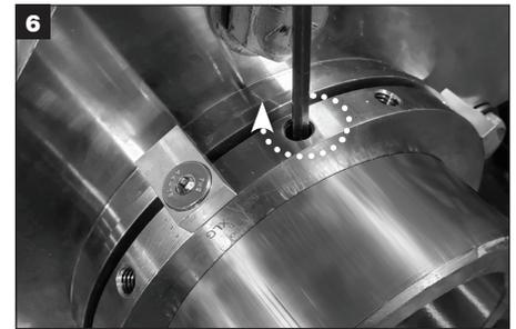
Tighten three dog point set screws ① (see inset image, marked with a dimple) evenly with the hex key provided.
