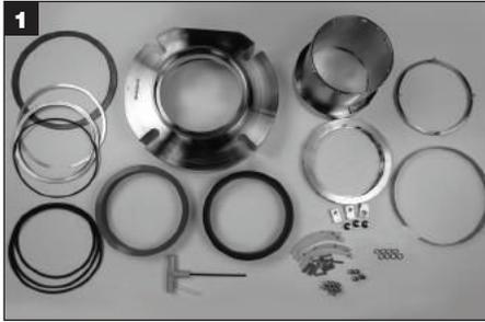
Tools required for assembly of seal: Hex key and two types of grease (supplied with seal); lint-free cloth, tweezers or a thin pick (supplied by customer); for installation of O-Rings and drive tube). Clean all metal components with an approved solvent, including all gasket and O-Ring surfaces. Place metal components and all spare seal components on a clean dry surface.
