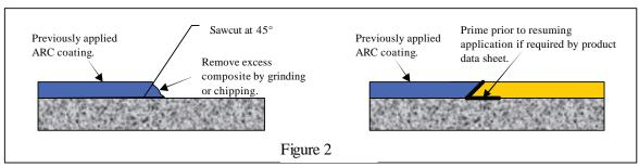
substrate, remove excess composite with a chisel, and reprime leading edge. Continue application (Figure 2).
