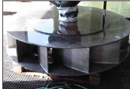
Hot water wash with grit blasting
