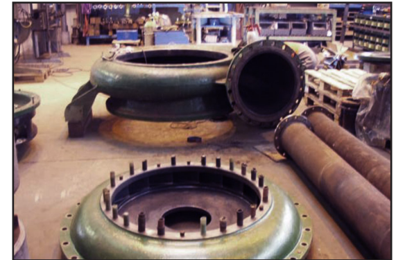
After 10 years of operation, the ARC 855 coating shows no damage
