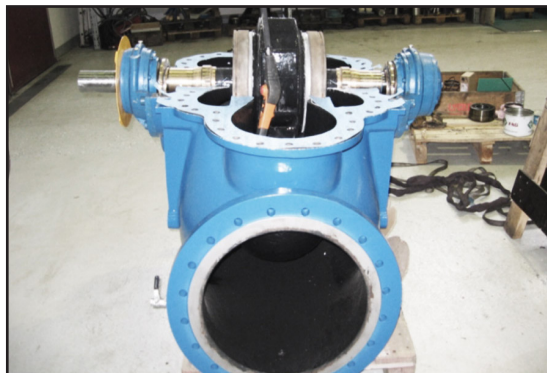
ARC coated surface after dynamically balancing of impeller
