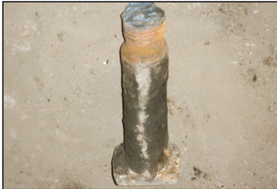
Customer originally applied graphite paste diluted with mineral oil.
