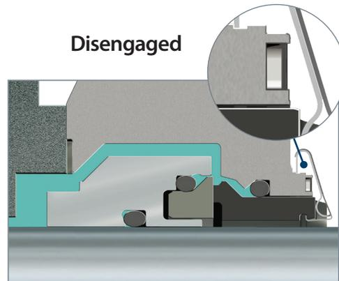
*After installation, the spring lifter automatically disengages while the gland halves are assembled, initiating spring force between the two seal faces.*
