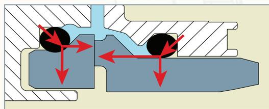
*Under vacuum conditions, atmospheric pressure acts on O-Rings, forcing them against the ramped surfaces of the seal faces.*
