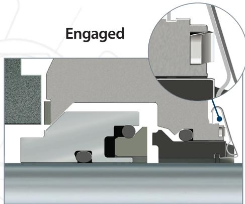
*The spring lifter is engaged and retracts the stationary face, providing ample space between the seal faces for ease of installation.*
