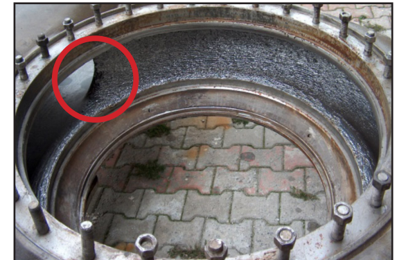
Casing after 12 months with ARC showing a small area requiring repair at the cutwater
