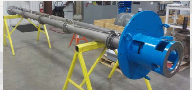
VS4 Sump Pump Repair
