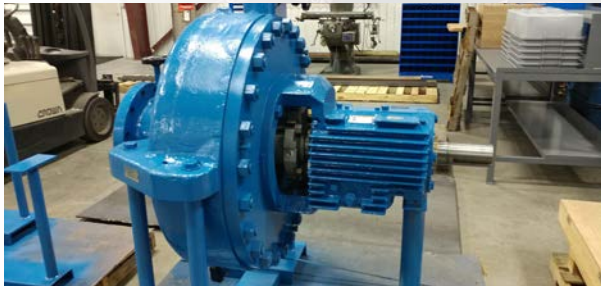
OH2 Horizontal Pump Repair
