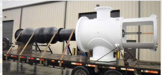
VS6 Vertical Can Pump Repair
