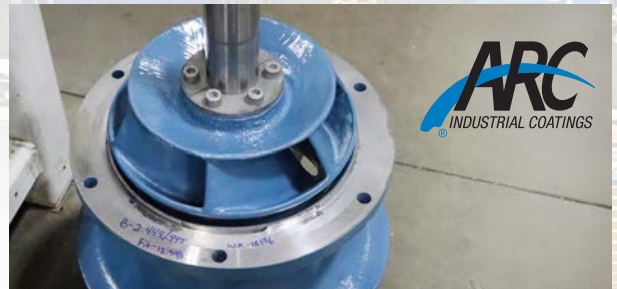
After – Repair of Pump with ARC Composite Coatings
