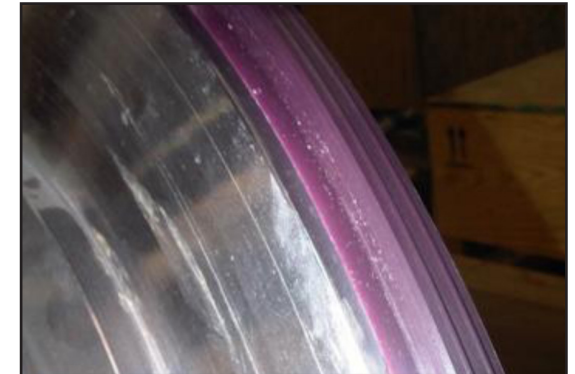
Seal shown installed onto the runner blade hardware.
