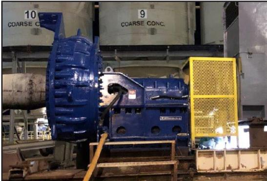
Figure 1: Large pump required adjustments every few days due to severe leakage.
