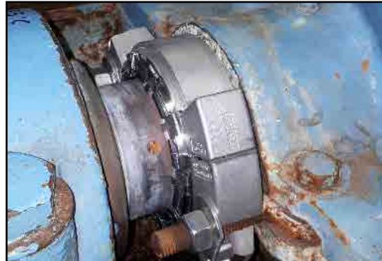
The 442C Split Seal was installed very simply.
